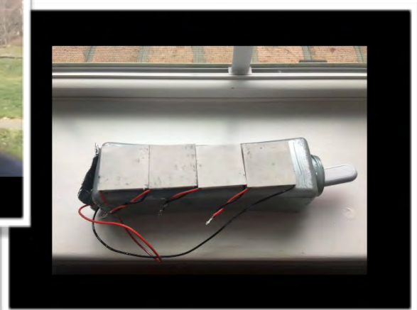
As part of their project, Abigail Xu and Emily Sun developed two prototype flashlights. This photo shows their second model made from a plastic water bottle lined with aluminum foil and covered with four Peltier tiles for heat transfer.
